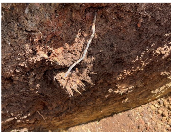
Wire and timber encountered in TP-S2.
