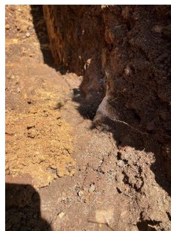
Broken concrete encountered in TP-S1.
